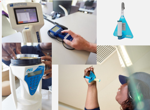
Punctual IAQ audit held by Veolia using precision measurement instruments (CO 2 , CO, TVOC, RH, T, PM, biological contaminants, Benzene and Formaldehyde)
